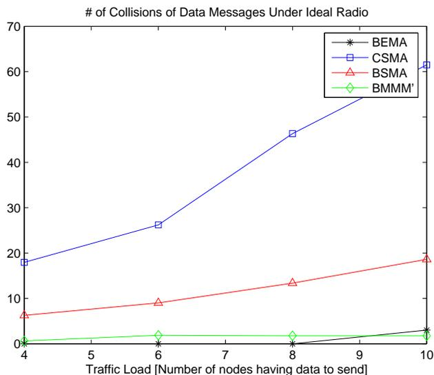
Figure 6. Collision in ideal radio model.
