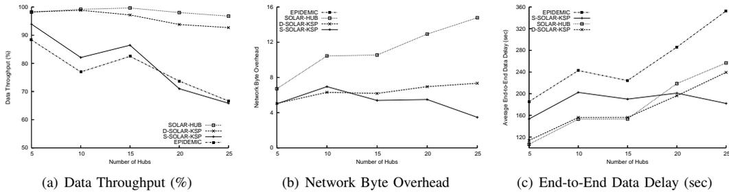
Fig. 7. Protocol Performance vs. Number of Hubs
