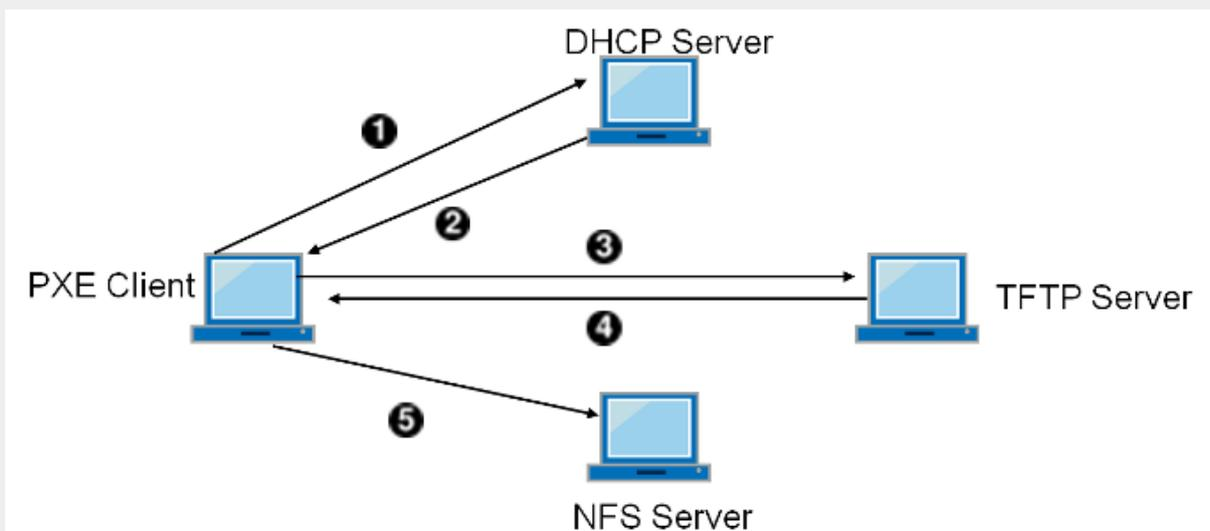
Figure 78. PXE Booting Process with NFS Root Mount
